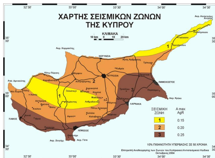
Figure 9: Values of the peak ground acceleration for a PoE of 10% in 50 years, as used to define the design spectra of EN1998 for Cyprus
