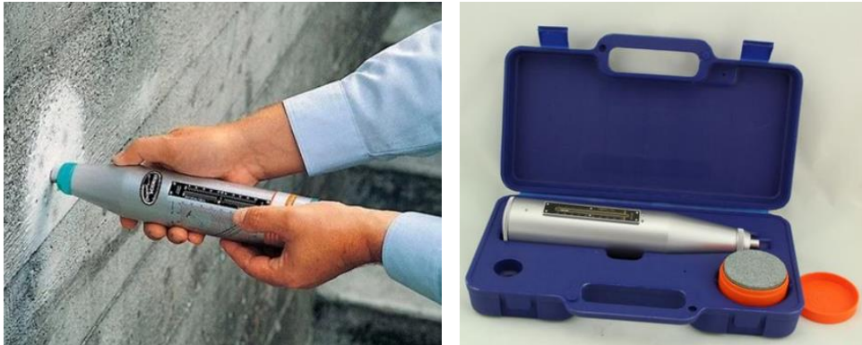
Figure 5: Schmidt Hammer Rebound
